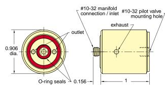
Type: 3-Way Normally Closed, Pressure Piloted Valve
