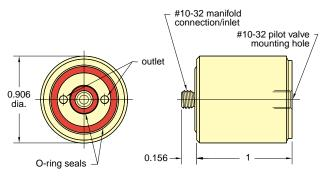
Type: 2-Way Normally Closed, Pressure Piloted Valve
